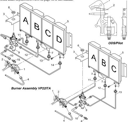
**Burner Assembly VP16ITA**
